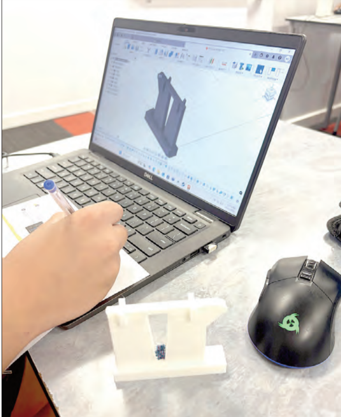
• This Year 8 student was introduced to the Fusion 360 CAD design program in Year 7 in TED in 2024. Currently on prototype number 10, he has created a resistor holder that has a hinged lid and securely closes for the safe transport of these small electronic components in his pencil case.
